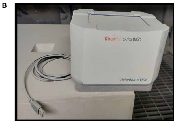
Figure 1. Images showing the VisionMate HSX barcode reader in the dust chamber before/after testing for ingress of foreign objects. Note the talcum powder covering the VisionMate™ HSX barcode reader after testing.
