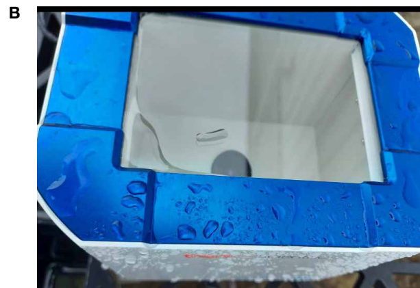
Figure 2. Images showing the VisionMate HSX barcode reader before/after testing for ingress of water. Note water in the up-close image after testing.
