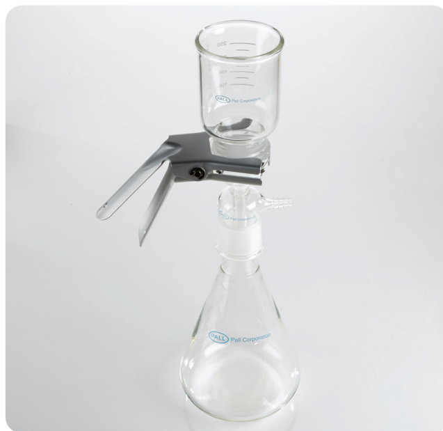
Figure 2: Mobile phase filtration apparatus
